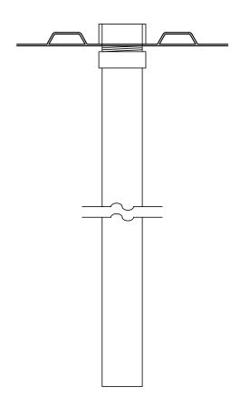
Available For 4', 6', 8', And 10' Diameter Tanks PVC Pipe To Within 6" Of Tank Bottom (Installed)
