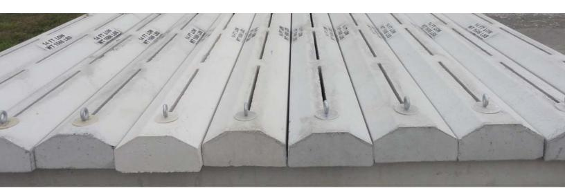
Containment Solutions offers pre-fabricated deadmen anchors and turnbuckles for all single-wall, double-wall and triple-wall underground fiberglass storage tanks. Deadmen anchors provide a means to prevent installed tanks from floating out of the ground when the tank installation is subject to ground water. Deadmen anchors are just as effective at preventing tank flotation but cost less than a concrete pad under the tank.
