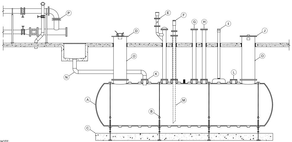
NOTE: All 6" FIBERGLASS FLANGES ARE FLAT FACED ANSI/ASME B16.5 CLASS 150, 25 PSI
