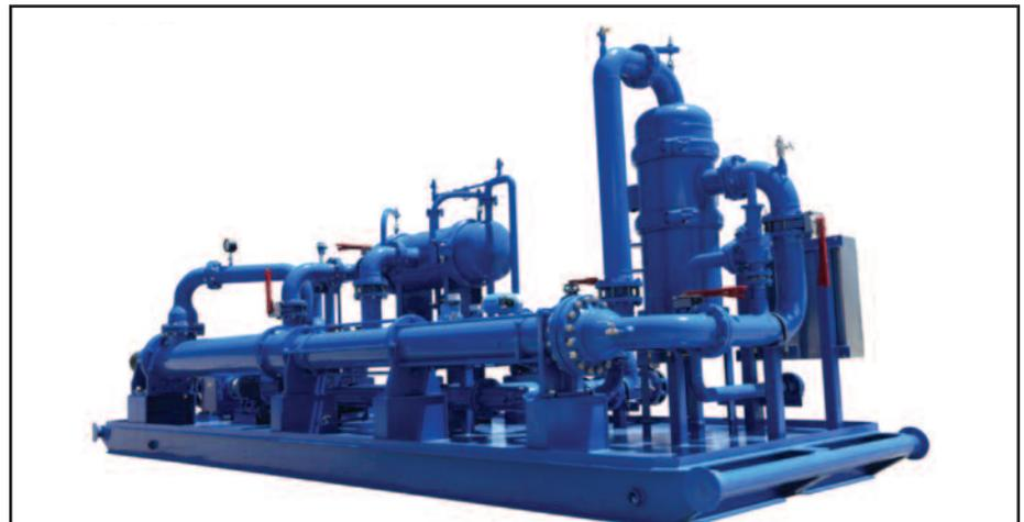
**The WaterWolf<sup>™</sup> Dynamic Oil Recovery system from National Oilwell Varco is designed to improve oil recovery from produced water while also reducing costs and solving HS&E issues. In addition to recovering oil, the system keeps gases under pressure and entrained in the water while removing suspended solids in a single treatment stage without chemicals. It can process up to 16,000 barrels a day per skid.**
