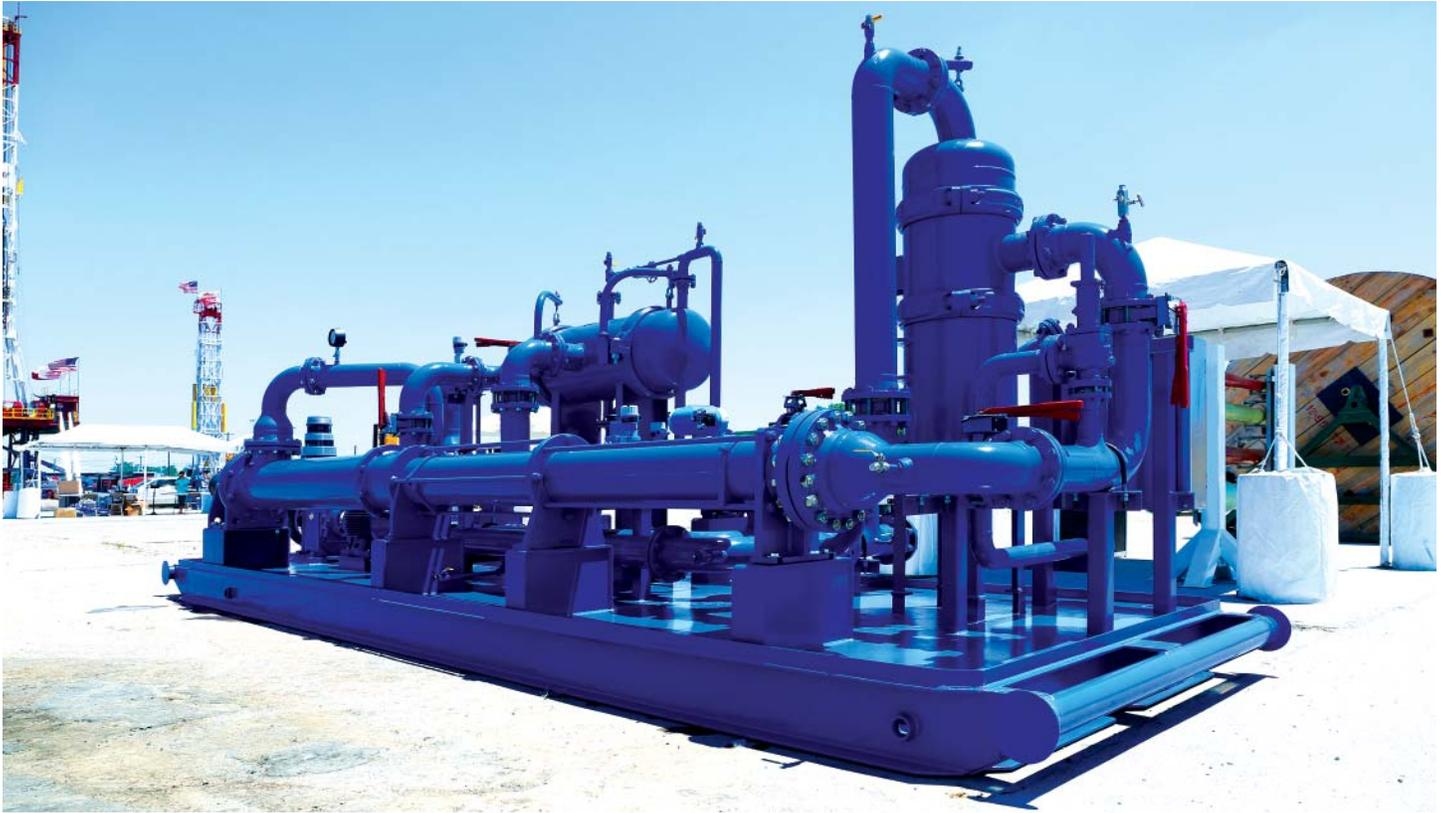
**SKID OPTIONS:** The WaterWolf Dynamic Oil Recovery system combines desanding and deoiling hydrocarbons with the non-shearing action of NOV's Moyno progressing cavity pumps.
